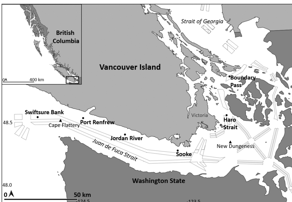
Fig. 1. Network of 6 passive acoustic recorders in the Salish Sea (black circles) and weather buoys at Cape Flattery and New Dungeness (black triangles) that provided wind reports. Locations of the international shipping lanes also shown (dotted lines)
