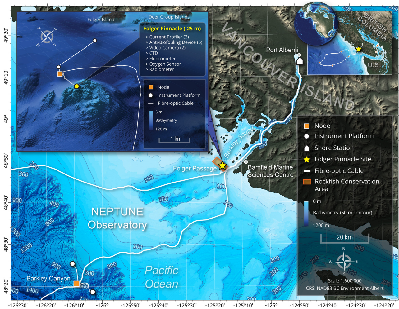
Fig. 1. Folger Pinnacle observatory location on the Pacific coast of Canada as part of the multi-node NEPTUNE fiber optic cabled observatory. Base map shows the study site positioned at the southwest entrance of Barkley Sound, on the west coast of Vancouver Island, Canada. Inset map (top-left) highlights the camera and multi-instrument platform location atop of the pinnacle at 25 m depth (textbox lists the equipment and number of devices on the Folger Pinnacle observatory platform)
