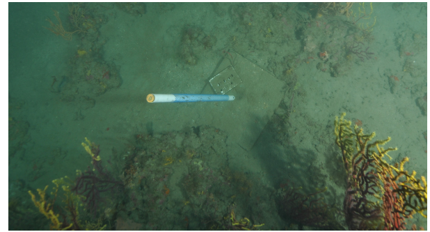
Fig. S1. Temperature sensor (left) and current meter (right) used to characterize the environment in the Catchoff site (Annex)
