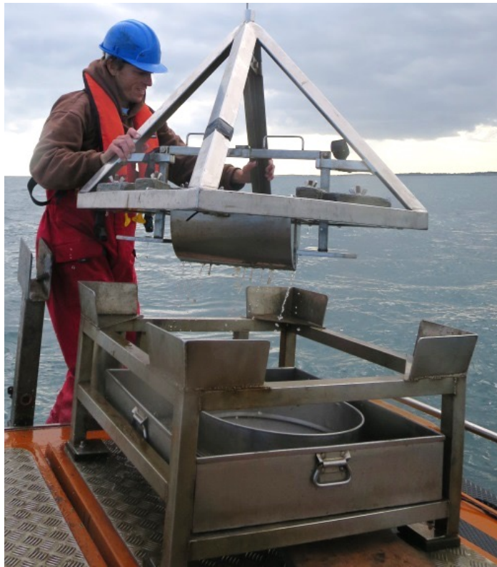
Fig. S1. Picture of the Day grab used to sample fauna. Photo credit: C. Bertolini
