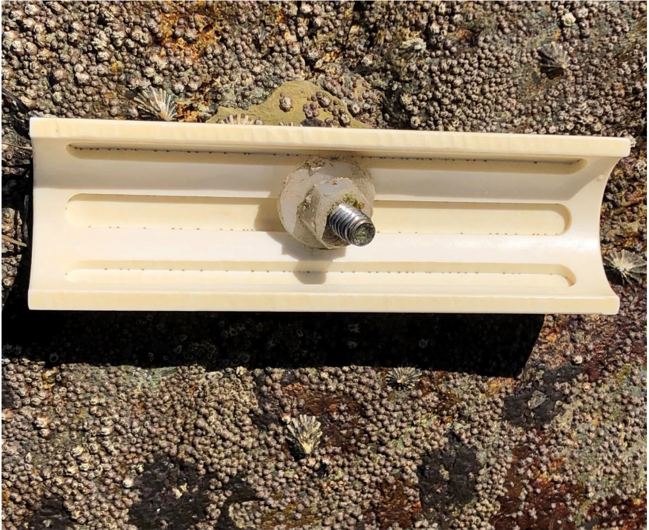
Figure S1. Settlement plate at low tide. Plates were made of polyvinyl chloride (PVC) pipes (11 cm long x 2.5 cm diameter), halved along the longitudinal axis with three grooves machined along the inner side. Plates were deployed in areas of dense adult Chthamalus fissus distributions (see barnacles in photo above and below the plate). Barnacle larvae typically settled inside the grooves of the plates (as shown above), except in instances of extremely high settlement. See Pineda (1994) for further description of plates and their implementation in monitoring barnacle settlement.
